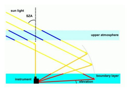
For each scan, several spectra (VIS and UV) at different elevation angles are measured.
