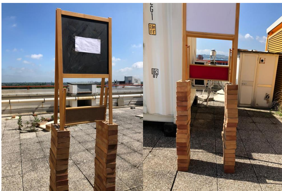
Figure B1: Left: Mala blackboard used for the white stripe elevation test (front view). Right: Mala blackboard used for the white stripe elevation test (back view) the Scanning Optical Device Collecting Atmospheric Light (SODCAL) platform can be seen in the background.
