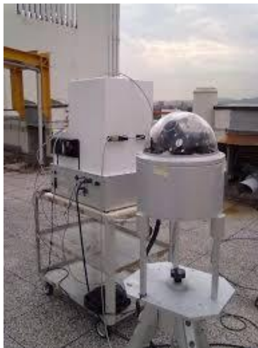
Figure 1: TROPOGAS instrument with Alt Azimuth platform on the CNR-ISAC roof in Bologna.
